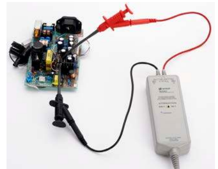
N2790A measuring a power supply signal
