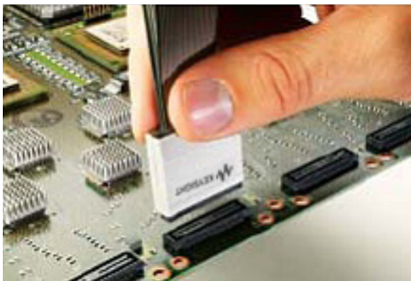
E5385A 34-channel Samtec connector probe
