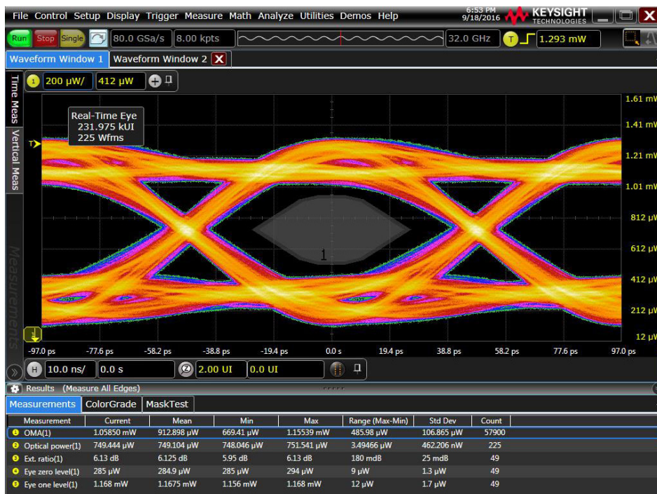
Figure 1. A full suite of optical measurement software is built into the Infiniium baseline software.
